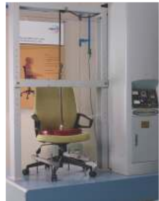
Testing of base for load bearing capacity
