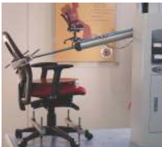
Testing of back tilt mechanism
